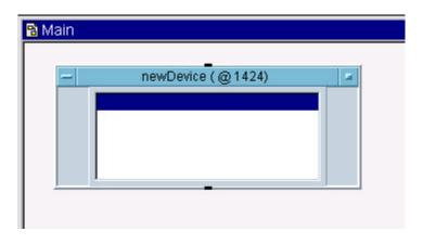
Step 5: Double click the highlighted blank line to add I/O transactions to this object. As shown below, we're sending the \*IDN? command to the instrument and then reading back the response with a string format. An output terminal has been added to the Direct I/O object.
